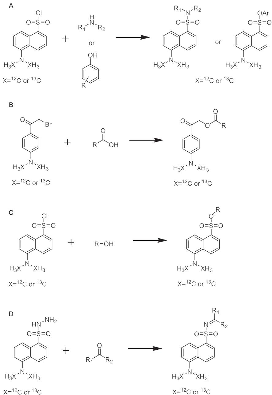
**Figure 2.3** Reaction schemes for high-performance CIL LC-MS methods. (A) Dansylation reaction for amine/phenol submetabolome. (B) DmPA labeling for carboxyl submetabolome. (C) Base-activated dansylation reaction for hydroxyl submetabolome. (D) Dansylhydrazine labeling for carbonyl submetabolome.
