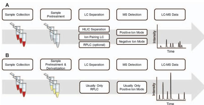
**Figure 2.1** Comparison of (A) conventional LC-MS method and (B) chemical derivatization LC-MS method for polar metabolome analysis.
